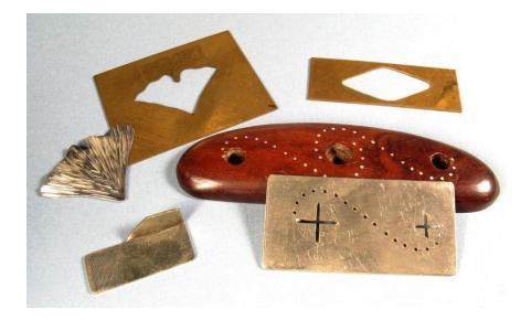
Whenever I have to make more than 2-3 exact copies of a sheet metal component, I think of making a template. Templates let me easily draw the shape of an item to cut out.
