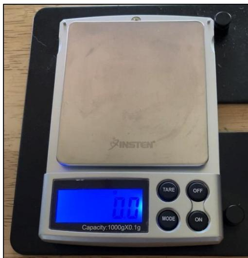
Figure 1. "Zero" the scale
