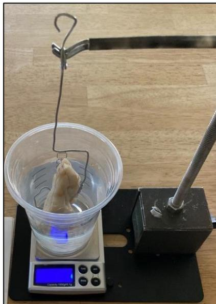
Figure 4. Record the reading on the scale. This is W, the weight of the mineral submerged in water.
